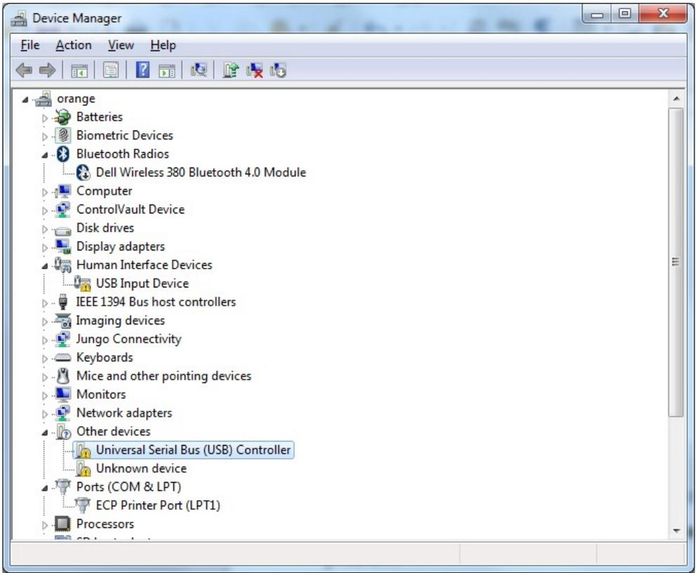
Either a new Universal Serial Bus (USB) Controller will appear (above), or JENCE CDC Serial Port 1.0 will appear (below)
