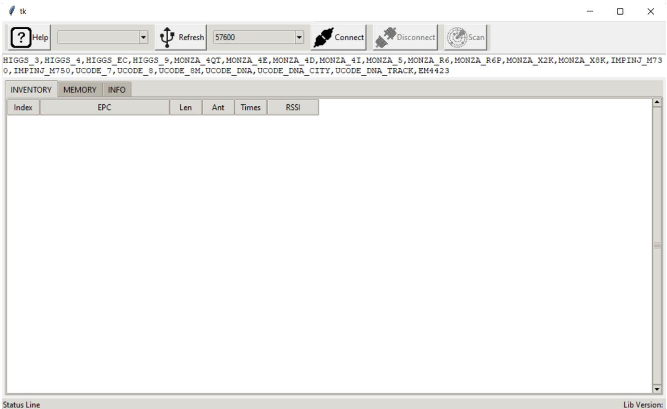
Please click on Refresh button and select the comport of UHF device (here, it is COM14). To connect the device please click on Connect button. If you place a UHF tag on the device and press scan button, the device will scan the tag and the unique EPC no of the tag will appear.
