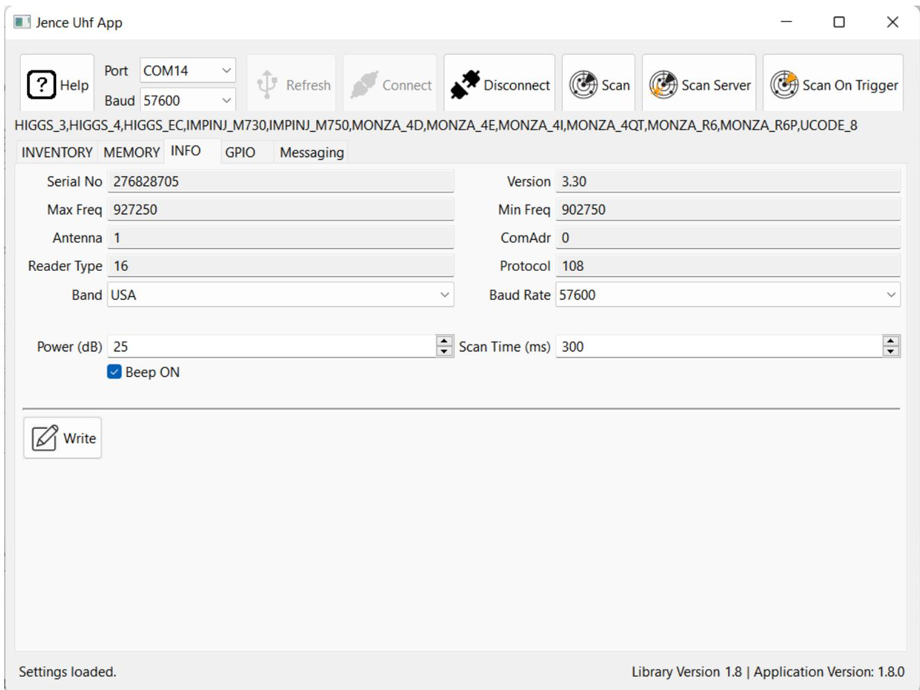
**Messaging tab:** This tab is useful for developers when they want the scanned data in JSON format. There are three ways to get JSON formatted message. The first option is send the JSON message to a Server Socket. In Windows, Cygwin and Linux or Mac OS X, `nc` command can be used to create a server with a single line.
